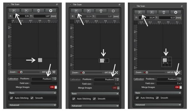
acquisition is completed, the images will be automatically stitched together to form a composite image.
