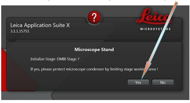
Software will ask for Stage Initialization, make sure the stage is moved downward & then press YES.
