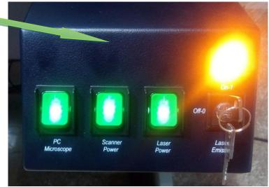
a). *First* switch on <u>*PC Microscope*</u>
