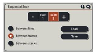
This option speeds acquisition of z-stacks but can result in movement artifacts and z-registration issues. These registration issues can arise if the z-focus does not return to exactly the same position for slice 1 of channel 2. This can cause errors, especially in colocalisation or ratiometric analysis.
